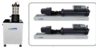
4. Cyclic Tri-axial Test - Used to determine the cyclic strength (sometimes called the liquefaction potential) of saturated soils
