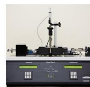
8. Direct and Residual Shear Test Device - To determine the Shearing strength of soil
