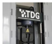
1. Cyclic Universal Testing Machine (Capacity: 600 kN) - Used for Rebar Testing
