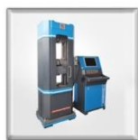
3. Universal Testing Machine (Capacity: 600 kN) - Used to test the tensile strength and compressive strength of materials
