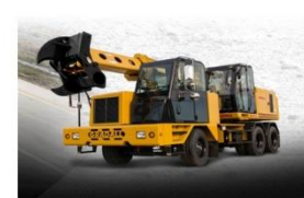
25. Cutter Crane with 30 inch slab cutting capacity & 9.65 ton lifting capacity - Demolishing RCC structure by cutting RCC/CC structures
