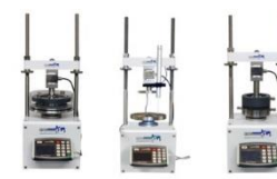
7. Automatic Consolidation - To measure the compressibility of soils
