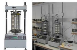
6. Static Tri-axial System - Determine of mechanical properties and shear strength of soil
