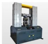
1. Cyclic Universal Testing Machine (Capacity: 600 kN) - Used for Rebar Testing
